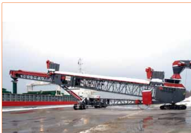
Layout showing Telestack's mobile materials transfer and ship loading system
