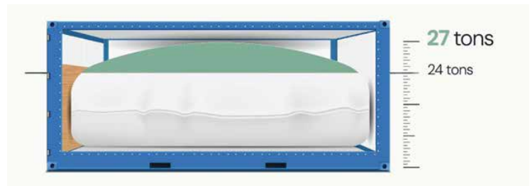
FIG 1. The AELER smart container can hold up to 27 tonnes of liquid in a flexitank.
